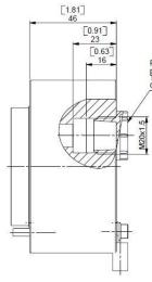
Plastic Screw Plugs are only for protection during shipping! They must be replaced by Ex d certified Cable Glands and/or Blind Plugs prior to use.
